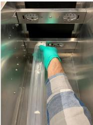
12) Put Bulb Clips over new bulbs and use screws to tighten Bulb Clips in place.
