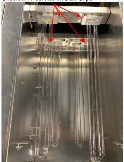
9) Carefully remove Bulb Clips and place aside.
