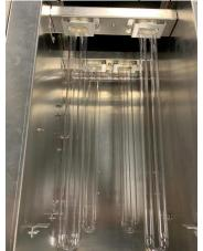
Replace Bulb Support Wires on top and bottom of bulb pairs. Use screws to tighten Bulb Support Wires in place.
