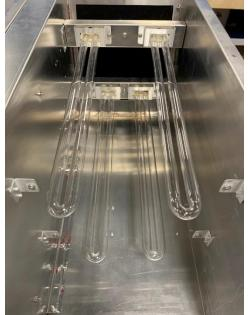
8) Unscrew <sup>1</sup>/<sub>4</sub>" screws on Bulb Clips.
