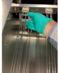
10) Remove all four bulbs by carefully pulling on the ceramic base.
