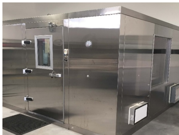
Figure 2: Bioaerosol Test Chamber Exterior.
